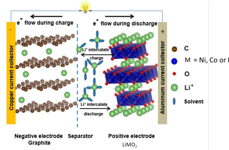
Lithium-ion cells contain a negative electrode, a positive electrode, and an electrolyte. As the cell is discharged, lithium leaves the negative electrode and moves through the electrolyte to the positive electrode. The reverse occurs when the cell is charged.
