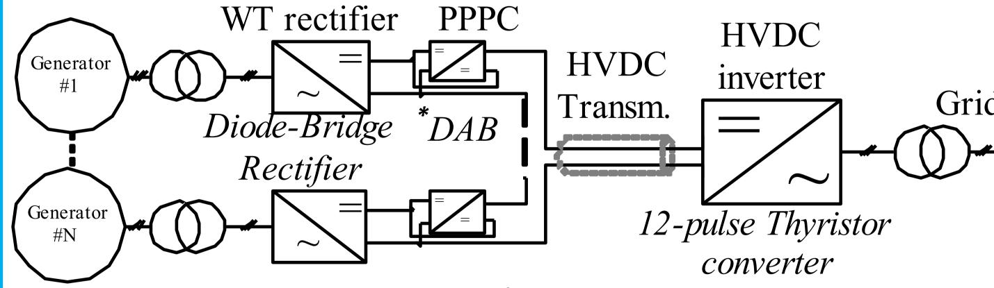
\* DAB=Dual-active bridge converter, an isolated DC/DC converter topology.
