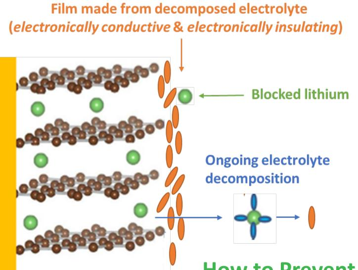
Parasitic reactions between the electrolyte and charged electrodes causes films of decomposed electrolyte to build up on the electrode surfaces over time. These films can block lithium-ions from entering the electrodes.
