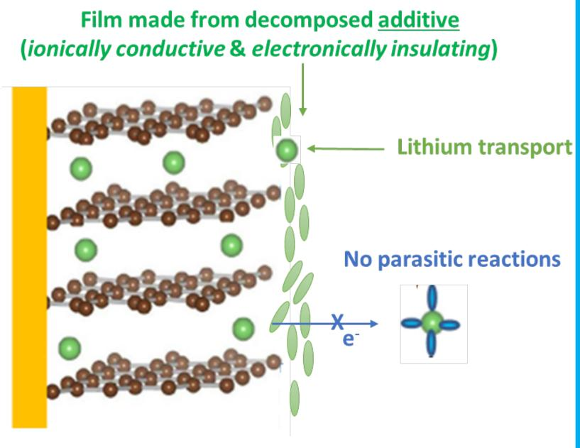
My PhD research is focused on: identifying parasitic reaction pathways, developing the best additives, and creating new techniques for analysing changes in electrolyte.
